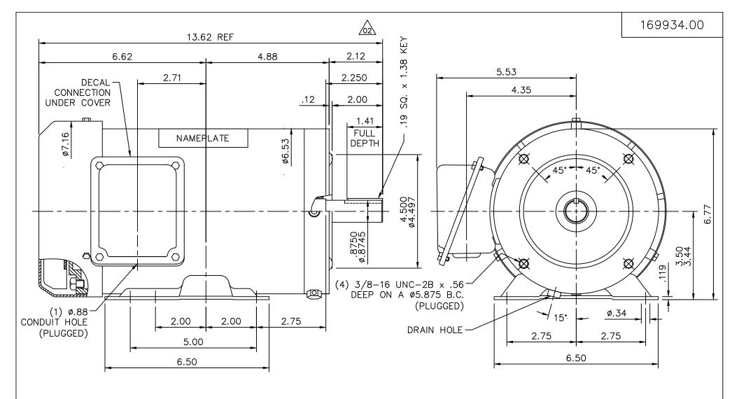
MAXIMUM FACE RUNOUT TO BE .004 T.I.R. MAXIMUM PILOT ECCENTRICITY .004 T.I.R. PERMISABLE SHAFT RUNOUT .002 T.I.R.
